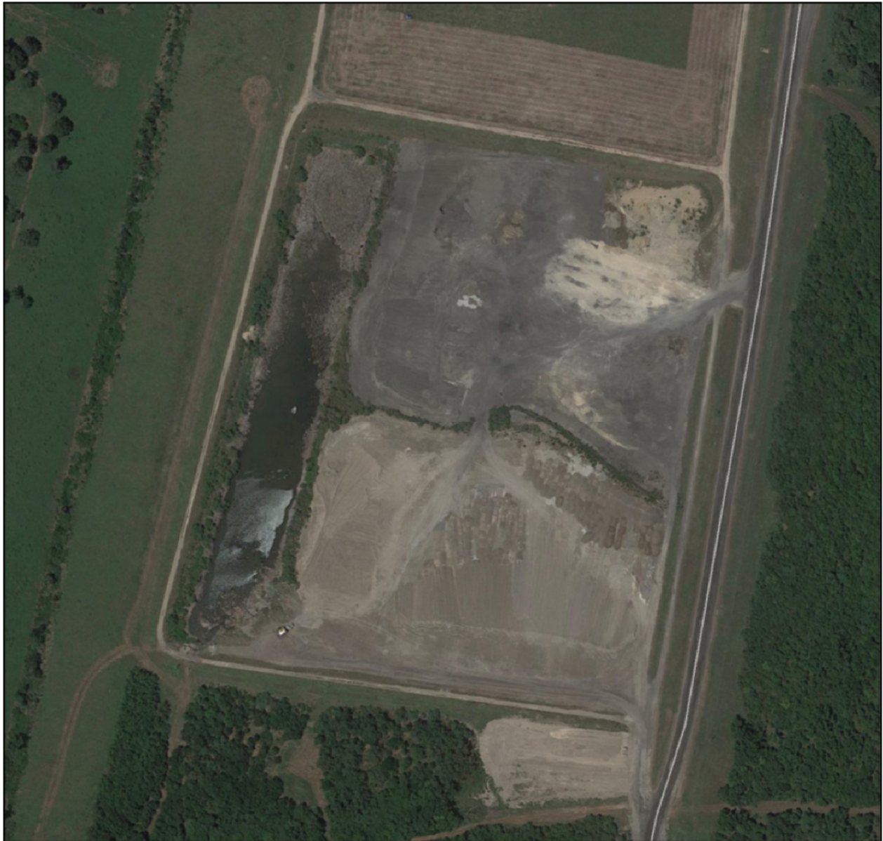
Photograph P-10 – From Google Earth Pro, dated July 2015. Downloaded January 8, 2016. Landfill Cell 3: Aerial view of Landfill Cell 3 and stormwater runoff pond inside western edge of Cell 3.
