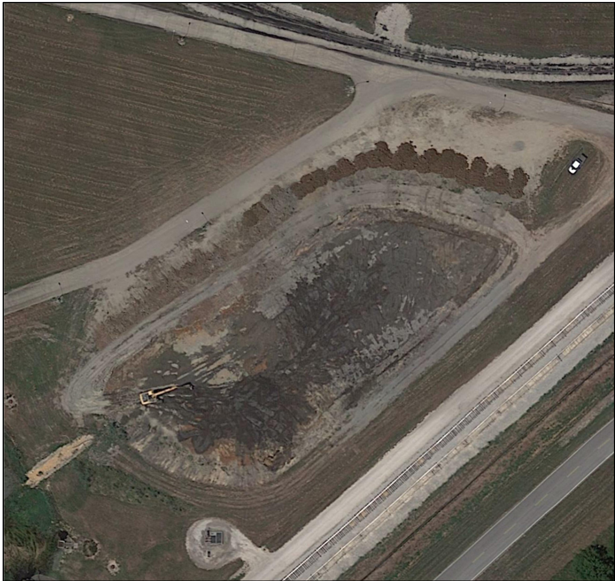
Photograph P-6 – From Google Earth Pro, dated July 2015. Downloaded January 8, 2016. Air Preheater Pond: Aerial view of Air Preheater Pond. Note pond dredging is underway at the time of the photograph. Also note the overflow channel from the western portion of the pond into the coal yard runoff pond to the west.
