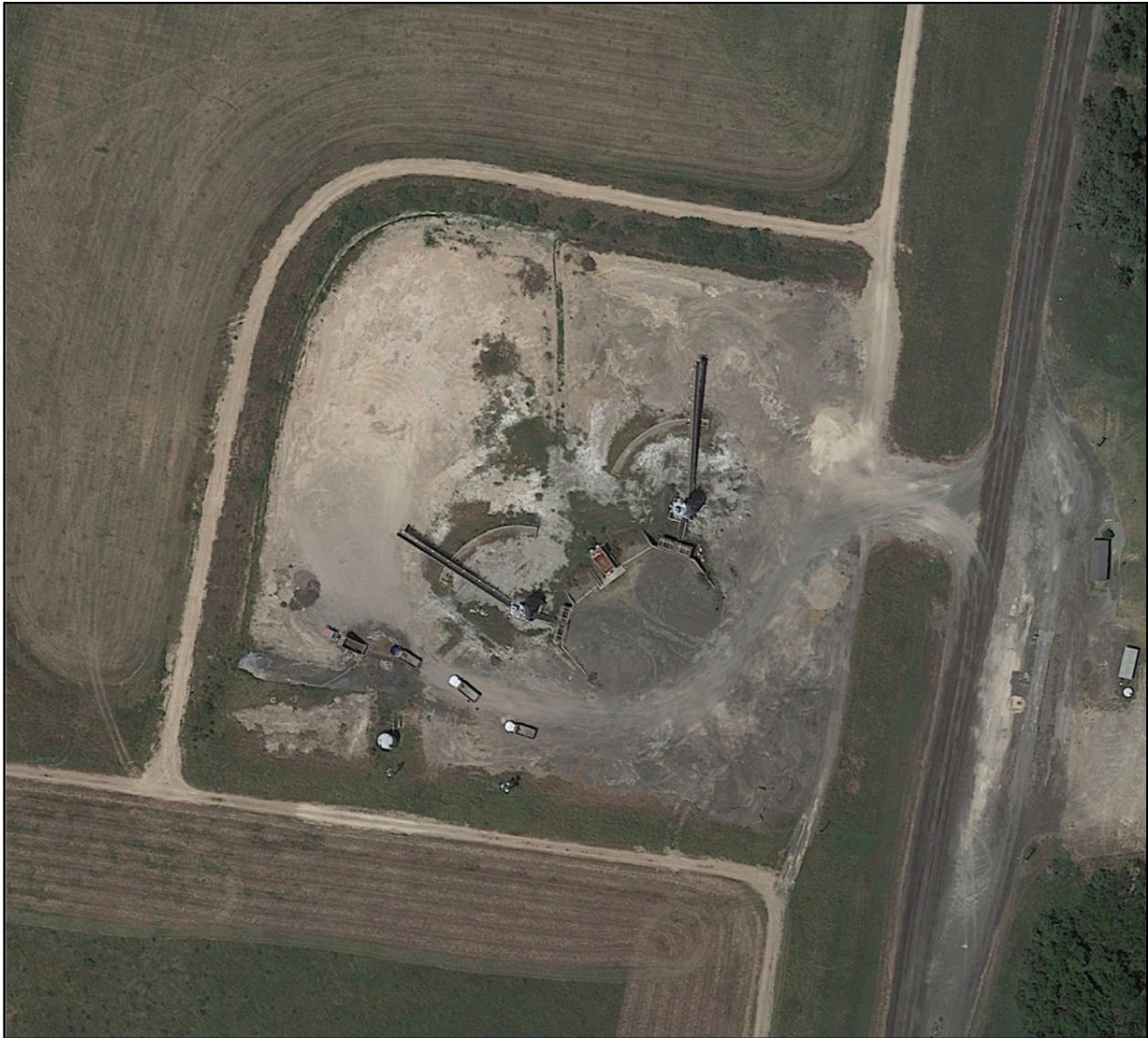
Photograph P-24 – From Google Earth Pro, dated July 2015. Downloaded January 11, 2016. Landfill Cell 2A: Aerial view of open area of Cell 2A, which contains a pugmill to stabilize CCR materials for disposal in other cells. The closed portions of Cell 2A are north and west of the active area.
