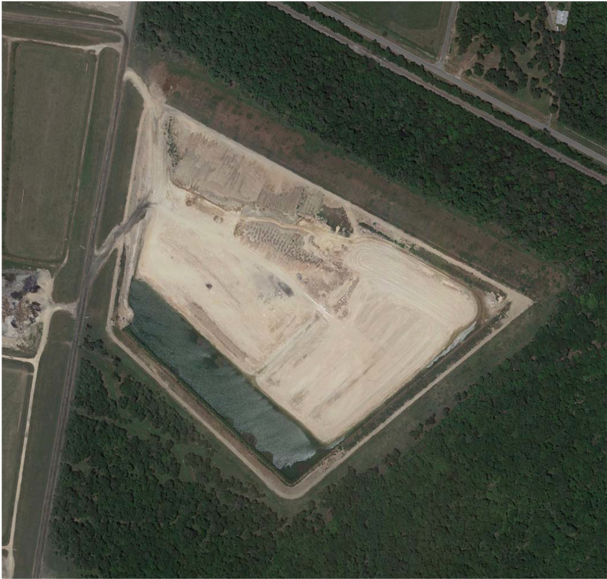
Photograph P-48 – From Google Earth Pro, dated July 2015. Downloaded January 11, 2016. Landfill Cell 2B: Aerial view of Landfill Cell 2B and stormwater runoff pond inside the cell.
