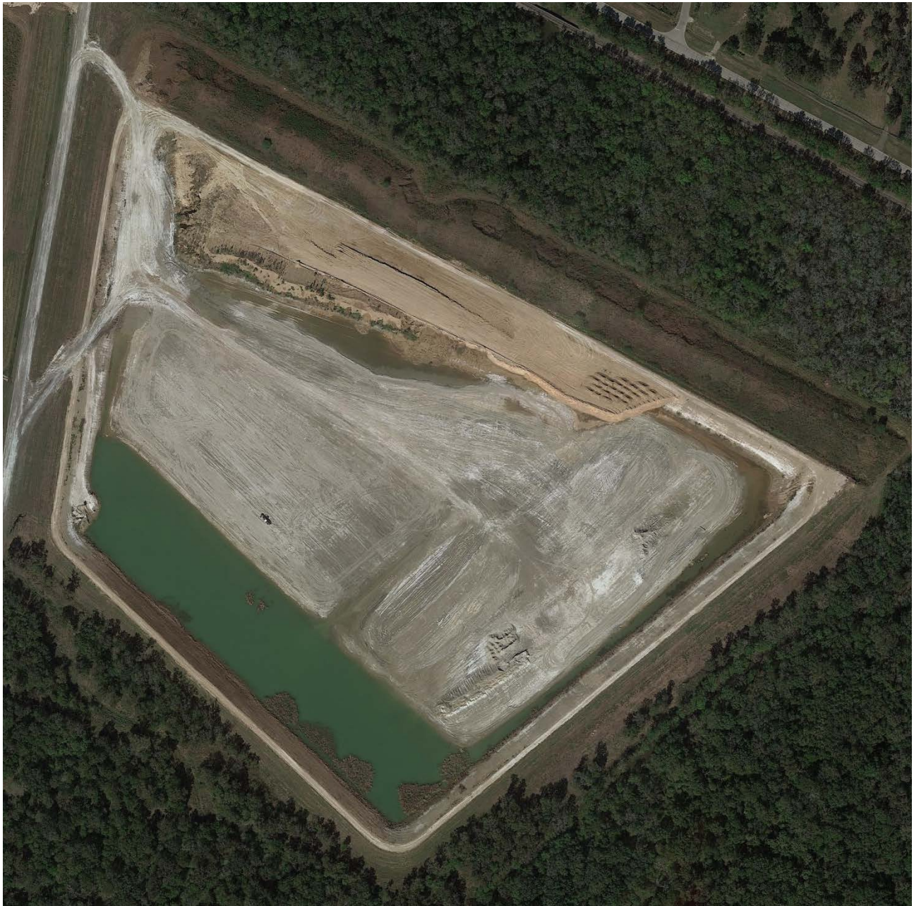
Photograph P-34 – From Google Earth Pro, dated October 28, 2017. Downloaded December 26, 2017. Landfill Cell 2B: Aerial view of landfill cell and storm water runoff pond inside the cell.
