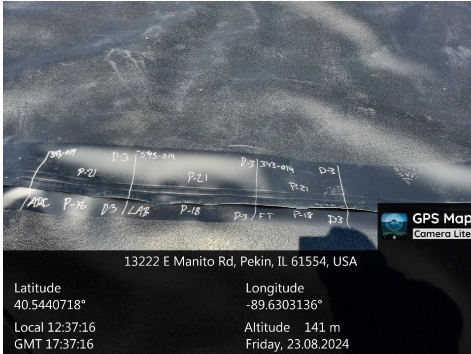
Photo 2: destructive sample D-3 laid out on panel seam P-21/P-18.
