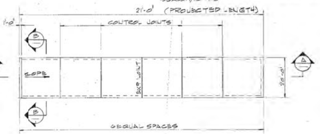
PLAN RAMP FOR METAL CLEANING BASIN (REF DWG 5080 C 5007) SCALE: 1/8"=1'-0"
