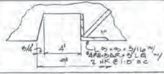
STOP PLANK GROOVE DETAIL EL. 465.6 SEE DET. A
