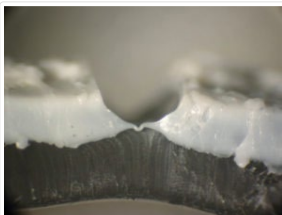
FIGURE 5 Photograph from 2014 of original razor-blade slit that extended through the white surface into the VLDPE core. During the NCTL stress-crack test, the sharp notch eventually blunted and did not propagate, which is a testimony to the functionality of the VLDPE core to resist stress cracking. No photographs were taken in 2018, but the NCTL results indicated continued very strong performance for this test.
